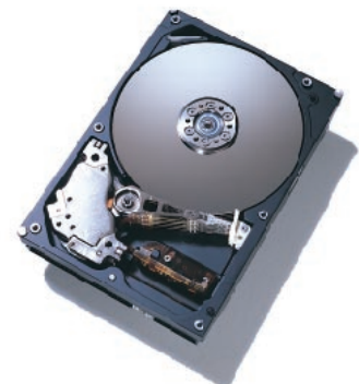
IBM Deskstar 60GXP 3.5-inch 7200 RPM 60, 40, and 20 GB ATA disk drive
