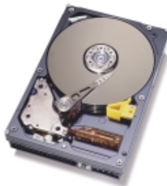
IBM Deskstar 37GP 3.5-inch 5400 RPM 37.5, 30.0, 22.5, and 15.0 GB low-profile ATA disk drive
